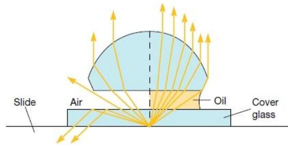
Fig. 8. Passing rays through dry and immersion objective (Prescott, 2013, adjusted).
