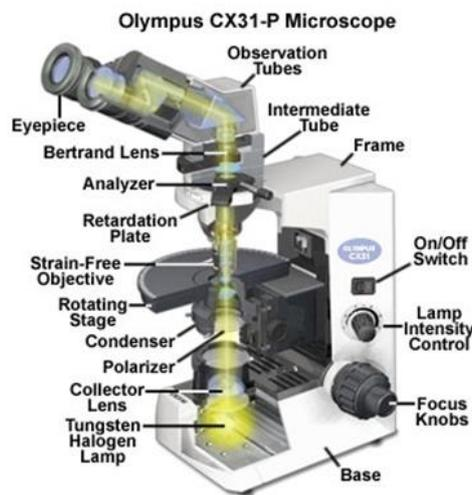
Fig. 7. Parts of the microscope (<http://www.olympusmicro.com/primer/techniques/polarized/cx31polconfiguration.html>, 12. 7. 2016).
